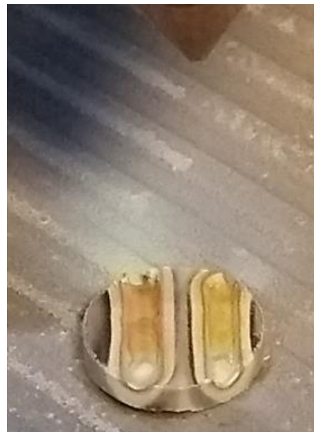
PZT Selective Laser Sintered
