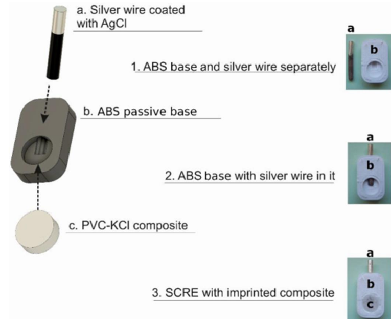
Fig. 2. Solid state 3D printed reference electrode. On the left-side a scheme with electrode parts; on the right-side fabrication steps and photos of a real product (dimensions of the base: 30 mm × 20 mm and cavity diameter 11 mm).
