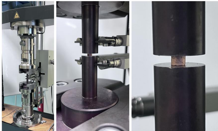
Test stand and sinter (before and after the compression test).
